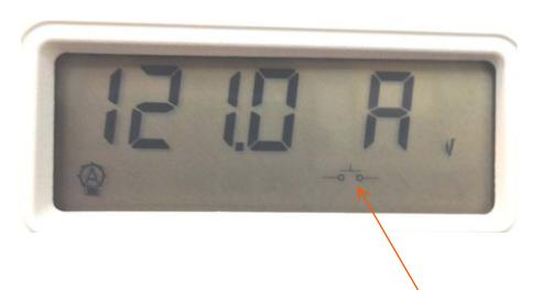
Switch in Open Position Irrigation Pump Disabled
