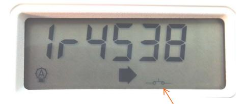
Switch in Closed Position Irrigation Pump can be turned On
